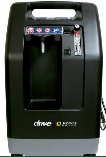
Oxygen Concentrator 10 LPM Model: Devilbiss Compact 1025
